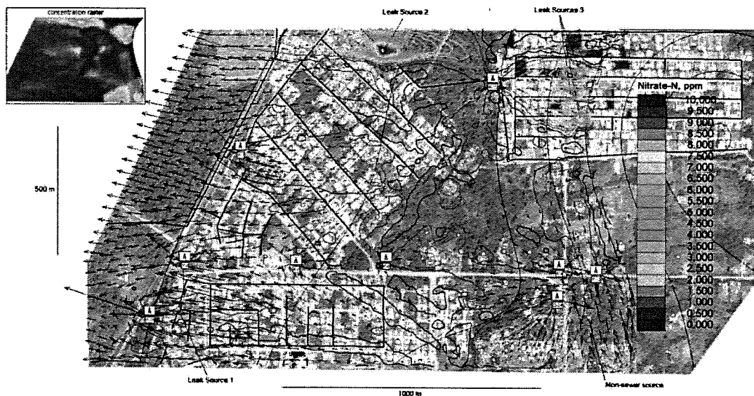
Nitrate-N transport from sewer leak scenarios and non-sewer resident sources, Machanao-Finegayan domain.
