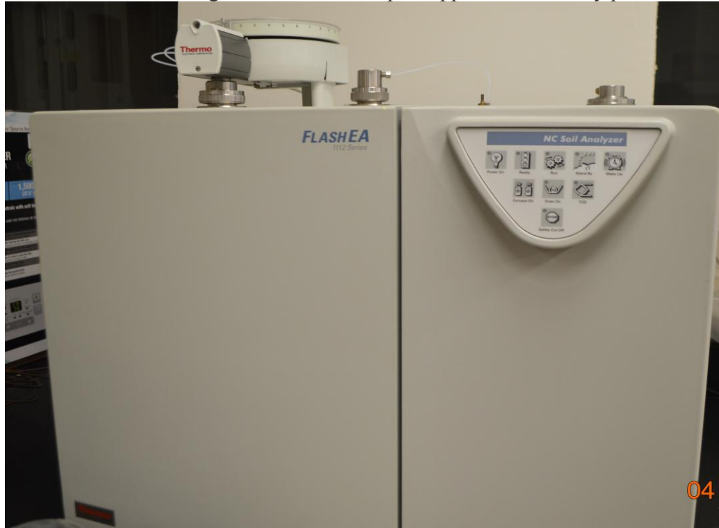
Figure 4: Nitrogen and carbon analyzer (FlashEA 1112 Series) used for soil and compost analyses
