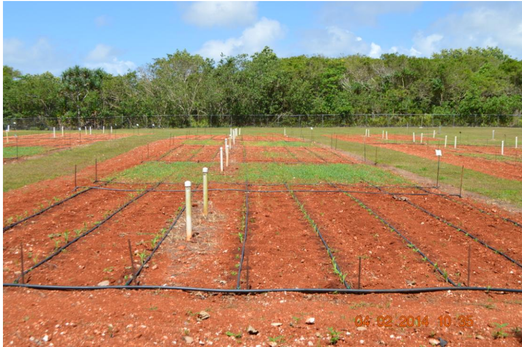
Figure 2: Study Plot Showing 8 rows of drip lines with 20 drip emitters per row at 1 ft. intervals
