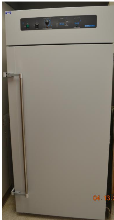
Figure 5: Shel-lab drier for obtaining harvested corn dry weight
