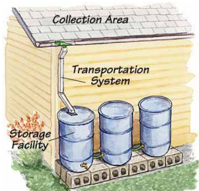
Figure 6. Diagram of a rain barrel system.
