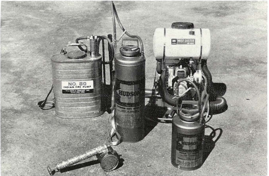
Sprayers come in many types, sizes, and price ranges. The spray gun or "flit gun" (left front) is usually sufficient for a small number of plants. For larger numbers of plants or in minigarden plots, the 2-gallon hand sprayer (right front), 3-gallon hand sprayer (center), 4-gallon backpack sprayer (left rear), or even the low volume mist blower (right rear) is recommended.
