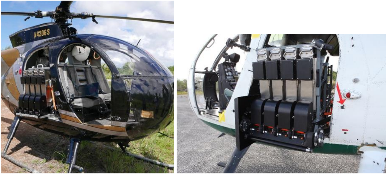
Image 3) The Aerial Deliver System (ADS) is made up of four magazines carrying 900 bait cartridges each, mounted on an OH-6 helicopter belonging to USDA-WS.
