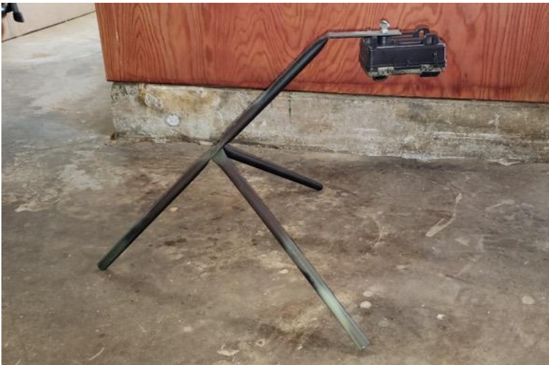
Image 5) Overhead-mounted game cameras were used to monitor fate of ground-deployed baits. The tripod was fashioned from electrical conduit pipe.
