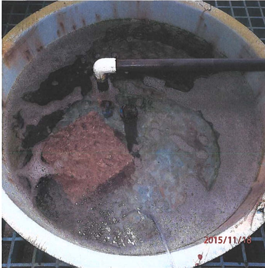
Figure 3: The tank set-up at the UOGML, supplied with a cement block, shade cloth, air, and fresh seawater from the flow-through system.
