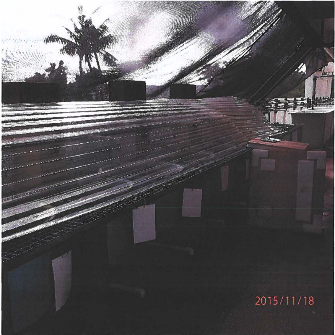
Figure 6: After dosing, the tanks were covered with a transparent sheet to prevent precipitates or foreign objects from entering the tanks and experimental information was recorded on water-resistant cards anchored beneath the tanks.
