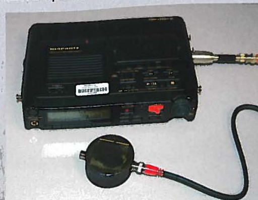
An early prototype of Moore's photosensor connected to a solid state digital recorder. This set up is used for field recordings of flying insects.
