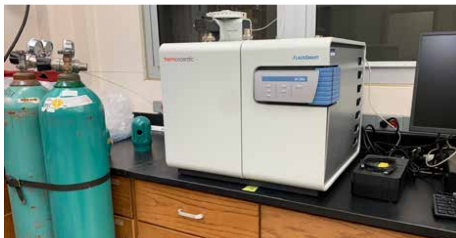
Figure 7. The Thermo Scientific FlashSmart Elemental Analyzer, located in UOG's Soil Lab, was used to determine total carbon (TC) and total nitrogen (TN) to evaluate soil quality.
