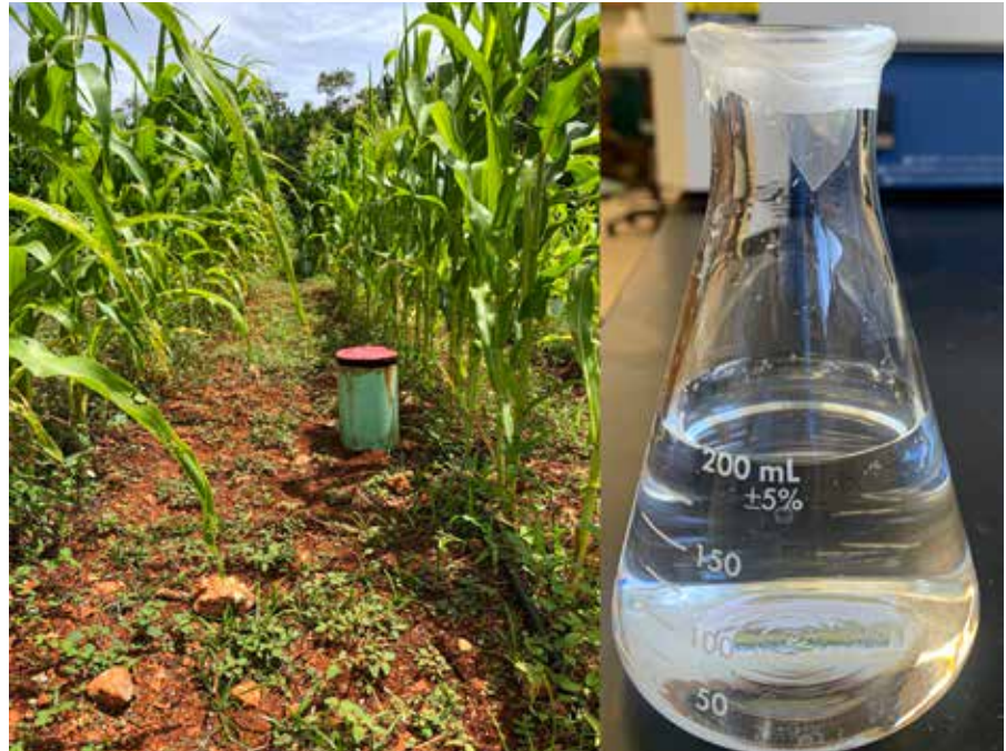
Figure 8. Sealed containers with 3M of sodium hydroxide-filled (NaOH) Erlenmeyer flasks were placed above the soil surface to capture CO 2 efflux in 24 hours.
