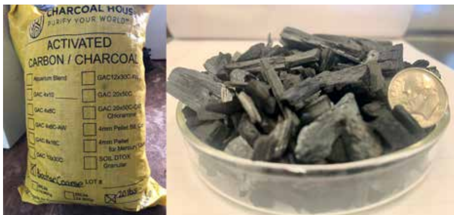
Figure 4. Biochar made from woodchips. The black color in biochar results from incomplete combustion, indicating high carbon content.
